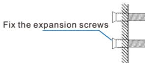
2. Fix the bracket onto the wall.
